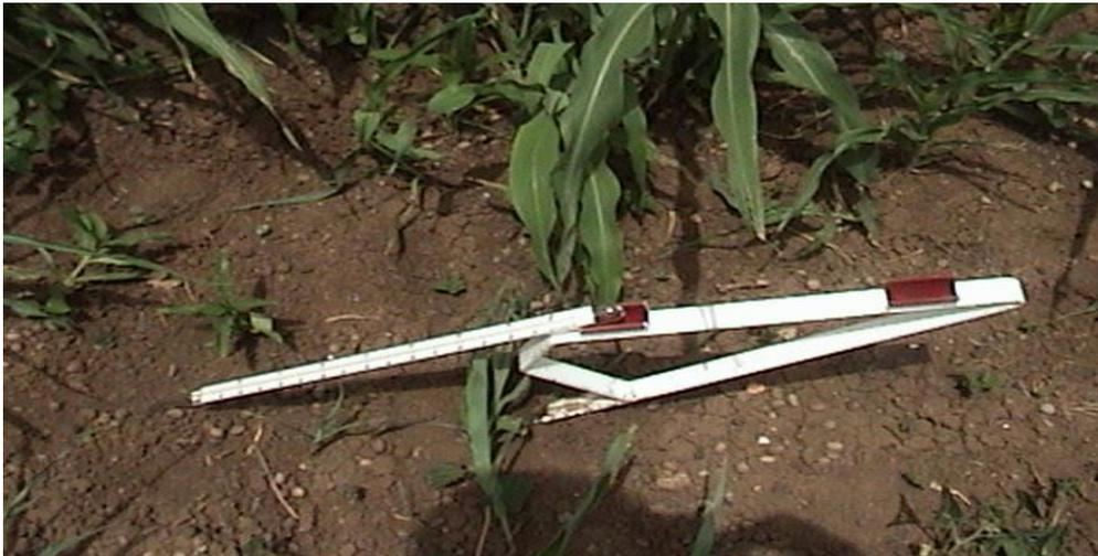
Photo (4): Soil temperature measurements, using soil thermometers at different depths, 5cm and 10 cm.
