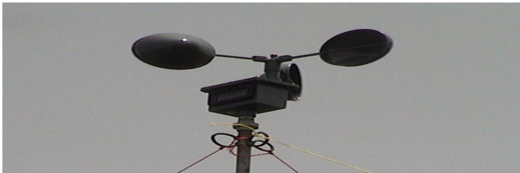
Photo (2): Cup anemometer, the instrument for wind speed measurement.
