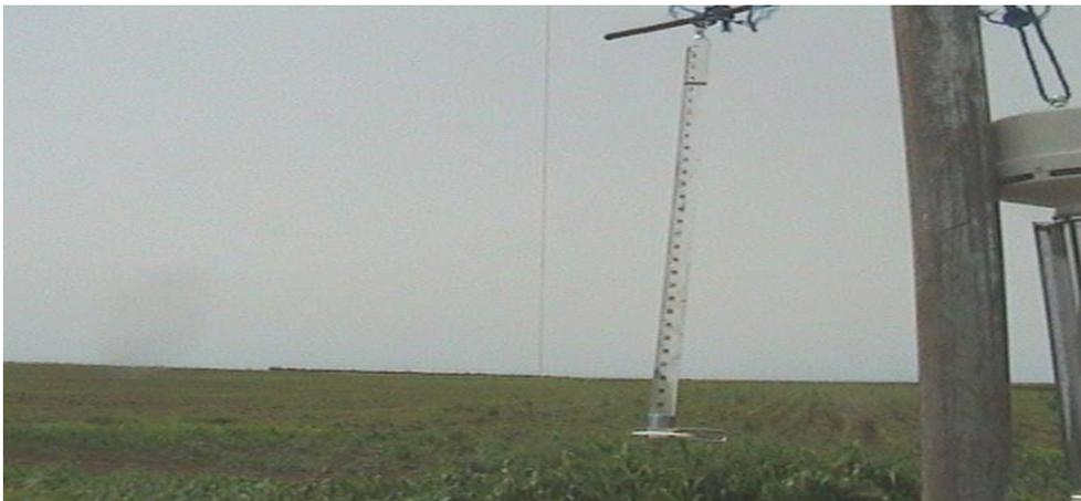
Photo (5): Piche tube used to estimate the amount of evaporation
