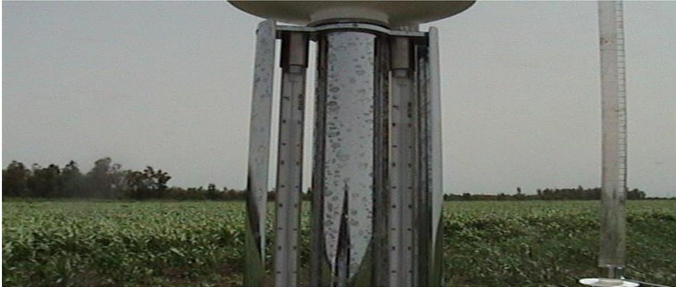
Photo (3): Dry & Wet bulb thermometers (Asamann), for measuring Relative Humidity, field work records, 2005 (El Faw shelterbelts).
