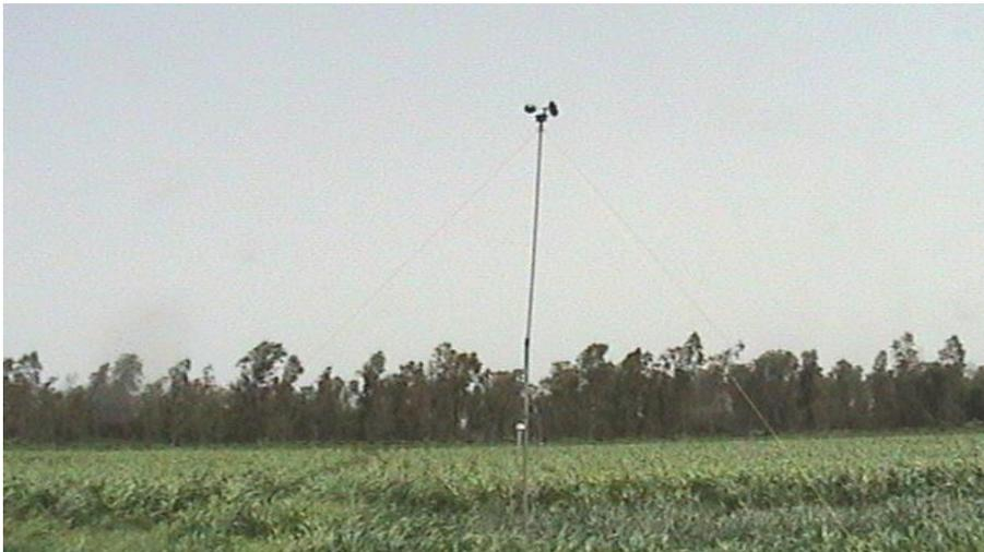
Meteorological station established at El Faw shelterbelt by the researcher during data collection for measuring some climatic elements.
